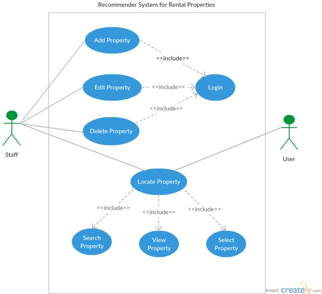
Figure 2: Use case Diagram for the Recommender System
